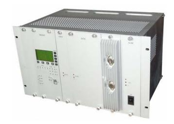
DPLC10 uses the high-voltage line between transformer substations as a communication path for the telephony and tele-control. This technology, which has been tried and tested over decades and adapted to the latest standards, has two main application areas: as a communications link between substations where a fiber-optic connection does not exist or would not be economically viable, and as a backup system for transmitting protection signals parallel to an installed fiber-optic link.
