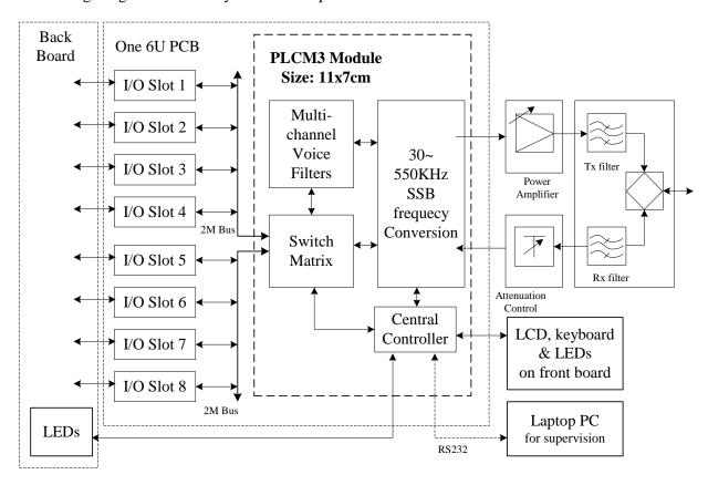
Each I/O slot is in common use for the following interface modules. The more I/O slots can be extended through E1 interface in another chassis.
